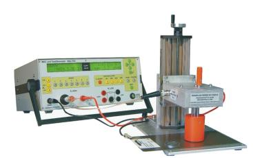
The measuring electrodes EH15/10 and EH15/20 are suitable for the measurement of volume and surface resistance atsmall pads.
