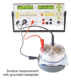
ring electrode in high-grade steel and aluminium quality
