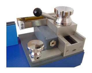
Die cable measuring fixture KMV 1000 was developed for measuring of the electrically resistance of cable-, wire- and other material specimens with an ohmmeter.
