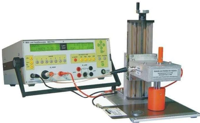
The measuring electrodes EH15/10 and EH15/20 are suitable for the measurement of volume and surface resistance at small pads.
