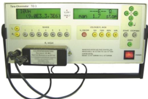
TO 3(optional) with High Ohm calibration resistor N8
