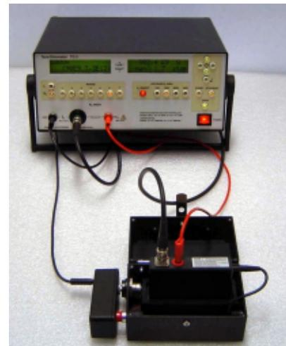
KB-HOW1 with HOW 1\*, calibration resistor\* and Milli-TO 3\* (\* optional)
