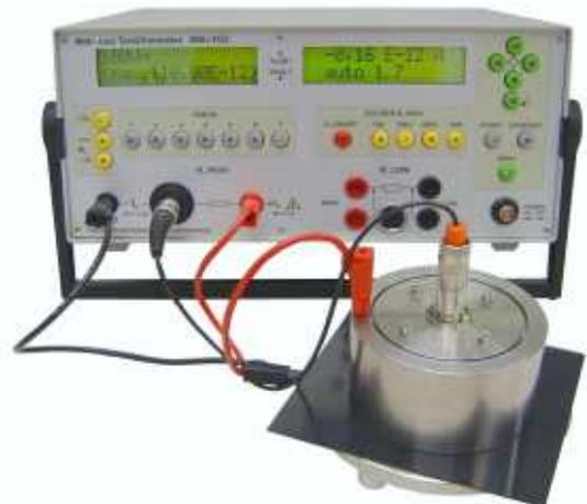
surface measurement with grounded baseplate
