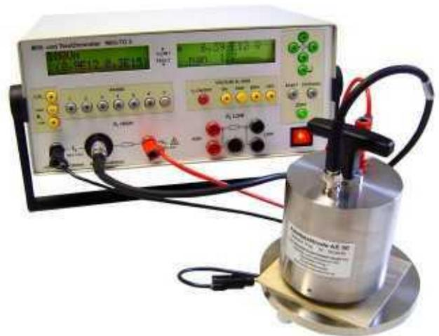
surface measurement with AE 50, grounded base plate GP 8.3 and Milli-TO 3 (optional)
