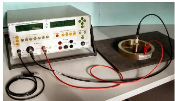
Measuring surface resistance with FGE 1 in connection with Milli-TO 3 (optional)
